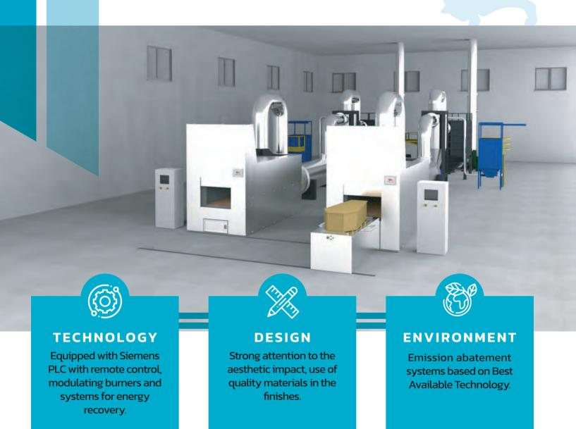
The FT crematory is a modulating type system with a hot hearth, therefore having a postcombustion chamber in the lower part and a cremation chamber on the back, with a wall and a sturdy sole built in refractory material with a high content of alumina on which the coffin will be placed, which divide the two chambers.
