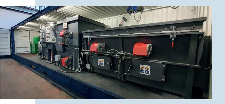
Our models of MB mobile incinerator ovens sare designed to be installed inside a container or on a trailer in order o be able to intervene immediately and directly on the waste production site, these incinerators are equipped with a fuel tank and energy generator and therefore can also operate in isolated places or disaster areas.
